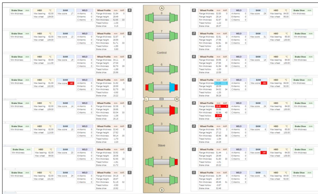
Figure 1: FleetONE unified data view of an 8 axle "coupled pair" wagon showing data from RailBAM, WCM, Wheel Profile, Hot Box Detector and Brake shoe imaging systems.
